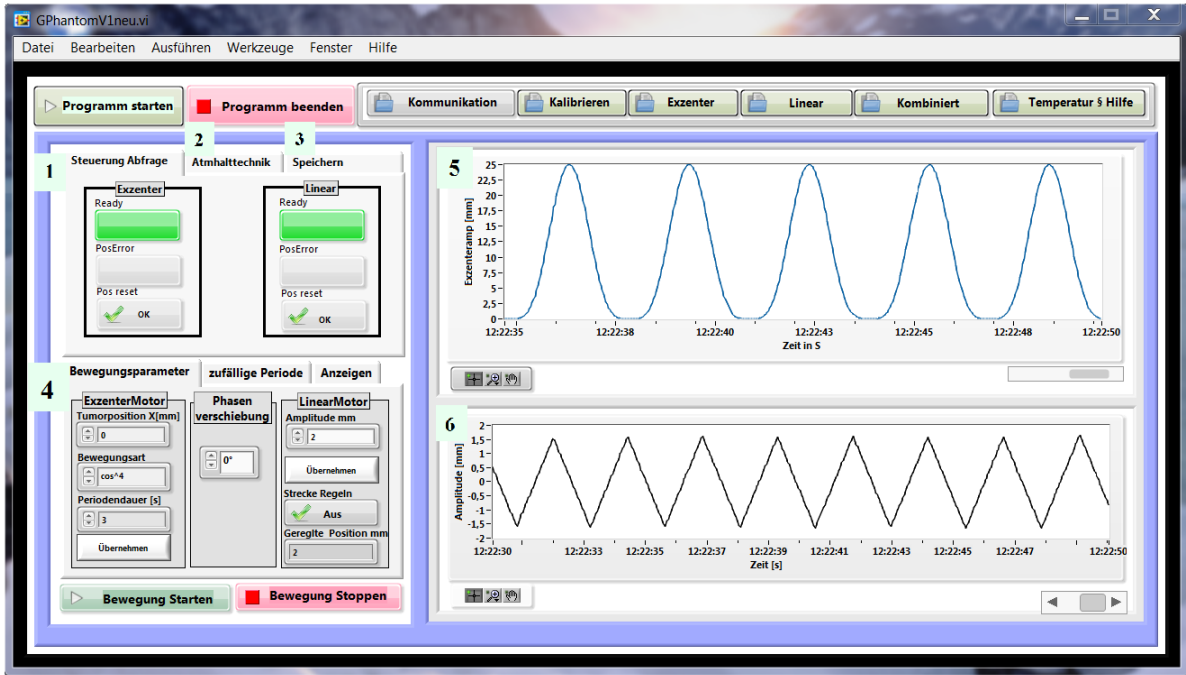
Figure 3.13.: Window Kombiniert (Combined): (1) Button to reset the position, (2) Breath-hold parameters, (3) Saving data parameters, (4) Bewegungsparameter (Motion parameters), (5) Eccentric motion curve, (6) Linear motion curve.
